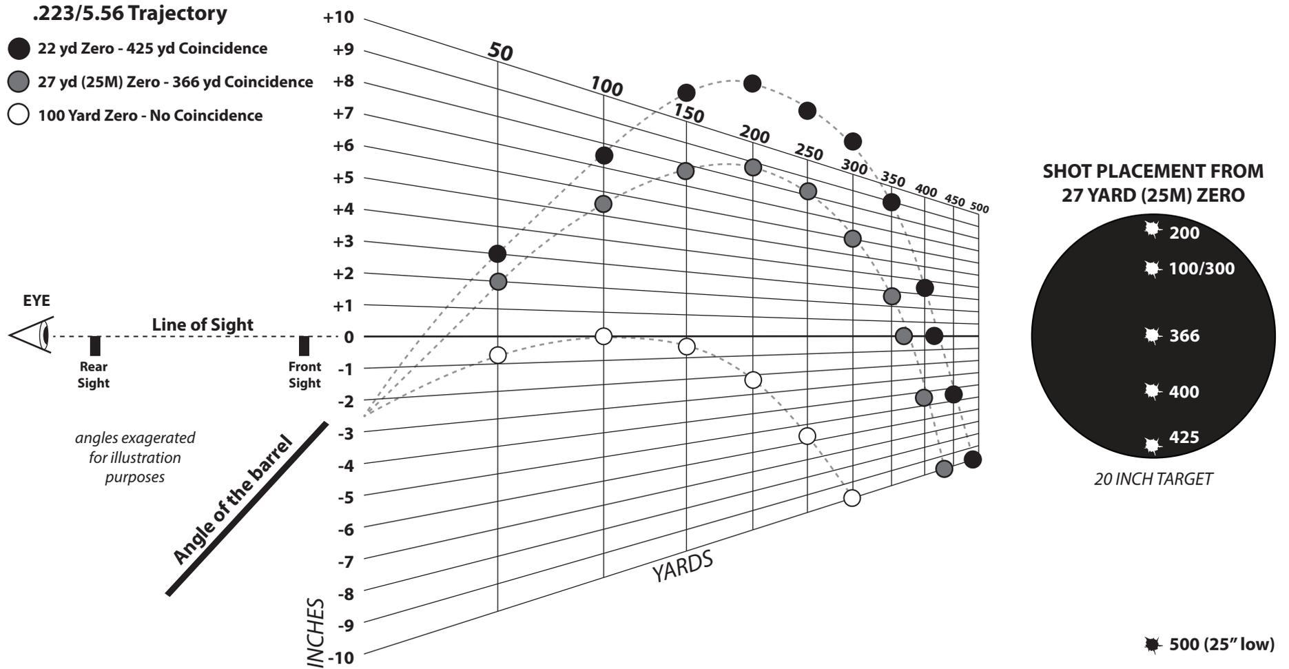
This chart is based on 16" barrel length, front sight 2.6" above bore, 55 grain FMJ @ 3080 fps.
