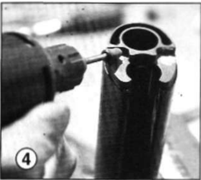
4 Grind the woodscrews flush with the surface of the middle band to provide clearance for reassembling the rifle.
