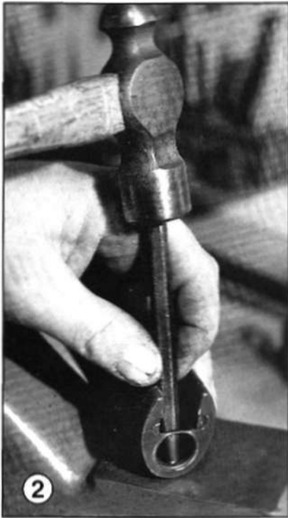
2 The barrel should not contact the front handguard. Peening the reinforce to clear the barrel helps achieve this condition.
