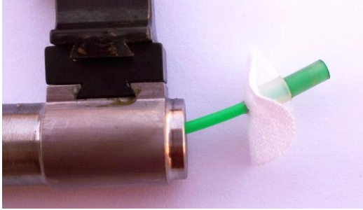
A dry patch started from the muzzle for cleaning the chamber after brushing with solvent.
