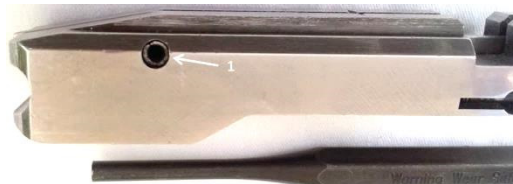
Stop pin must be pushed out with 5/32" roll pin punch
