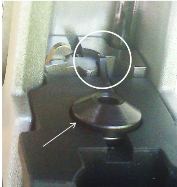
Bolt is locked open, magazine is out. Circle shows ejector protruding into recess to kick out round. Arrow shows magazine catch.
