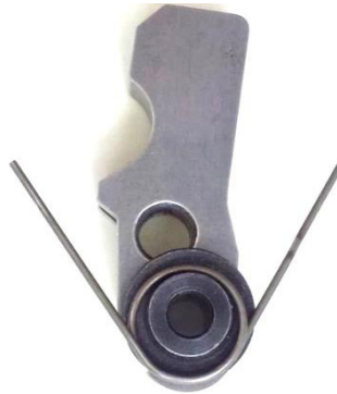
Right side of hammer assembly showing bolt lock spring installed on bushing. The dogleg of the spring is on the front side of the hammer.
