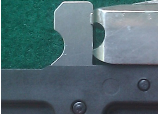
Bolt in battery allows hammer to rise to vertical. Note the overlap showing how little the firing pin protrudes from the bolt (bolt was placed slightly off centerline for this photo).
