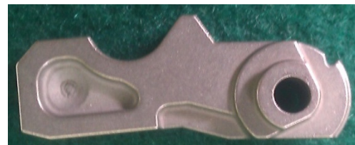
One-piece hammer does not require bushings.
