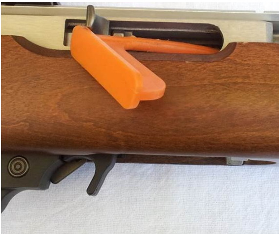
Flag incorrectly installed. There could be a round in front of the post.
