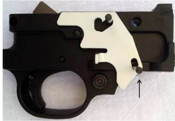
Press at arrow for “up” to lower lock Upper pin is now in front lobe
