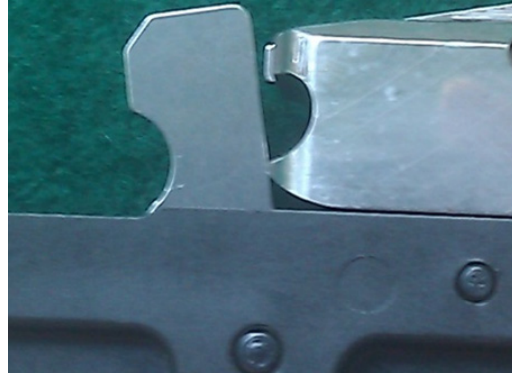
Bolt moved back a few 100ths of an inch. The hammer is caught on the lower edge and cannot reach the firing pin. This bolt was radiused by a professional.
