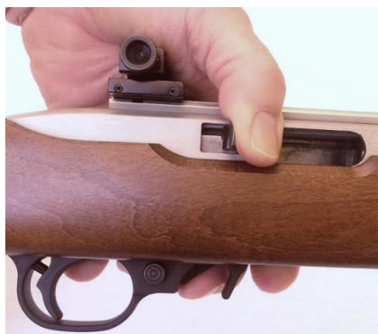
Left-handed bolt operation.
