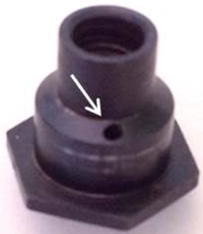
Hole in cap nut for spring tip
