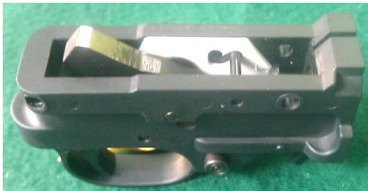
Bolt lock in lowered position, allowing bolt to glide over it. Pin is in front lobe of cutout. For this photo, the bolt lock is painted white, and the ejector removed. To lock bolt, pull it back, press the blade in and ease the bolt forward. Pressure from the bolt holds the lock in place.
