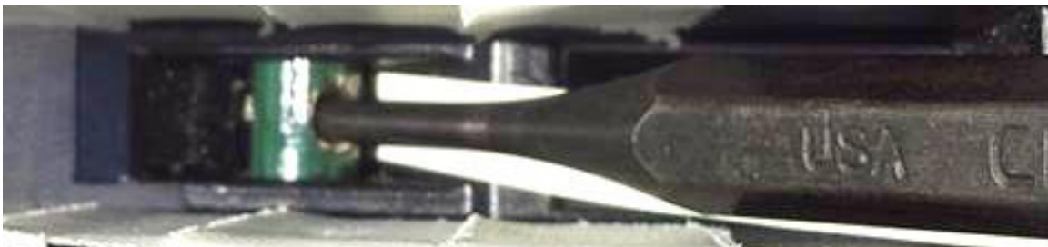
Tool is rotated so hole faces rear of housing to capture plunger underneath it
