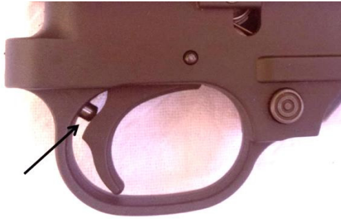
Arrow shows trigger return plunger
