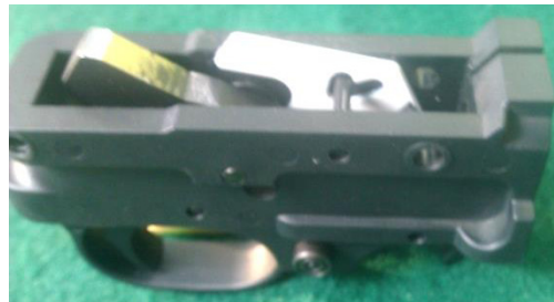
Bolt lock in raised position. Pin is in rear lobe of cutout. To lower it, pull the bolt back and press the forward part of the blade. The lock rises so that the point clears the pin, which then slides up into the front lobe of the cutout.
