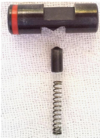
Safety, with detent plunger and spring.
