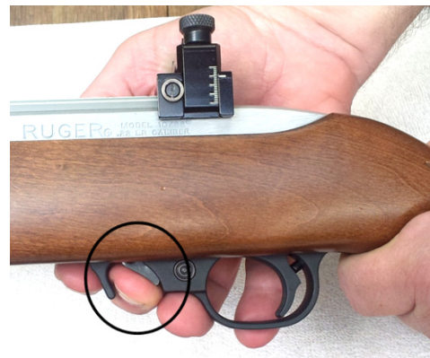
Finger presses lever while thumb holds bolt
