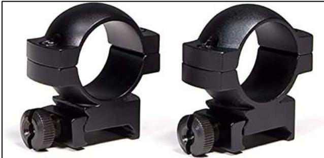
Parts called **rings** hold your scope firmly in place. The rings should be the same diameter as your scope tube. Vortex Optics offers a set of medium 1" rings (part number RING-M, pictured left) that will fit on the rail described above. Please follow manufacturers installation instructions regarding torque and thread locker.
