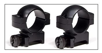
Parts called **rings** hold your scope firmly in place. The rings should be the same diameter as your scope tube. Vortex Optics offers a set of medium 1" rings (part number RING-M, pictured left) that will fit on the rail described above. Please follow manufacturers installation instructions regarding torque and thread locker.
